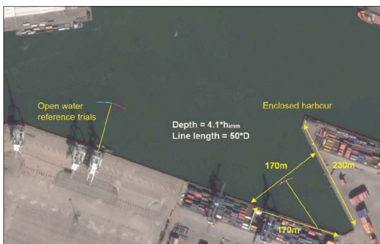
Figure 5: Sailed track of full scale validation trials under restricted environmental conditions
