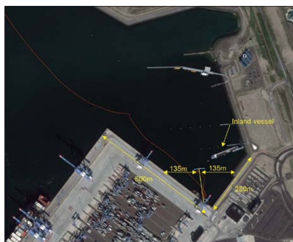
Figure 5: Sailed track of full scale validation trials under restricted environmental conditions
