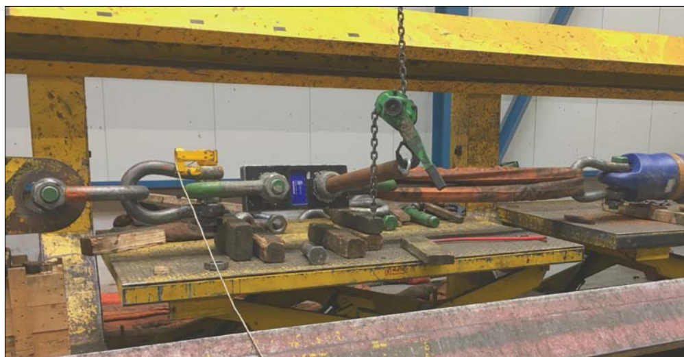
Figure 4: Systematic tests with load cells to evaluate effect of torsion when using steel stranded towlines
