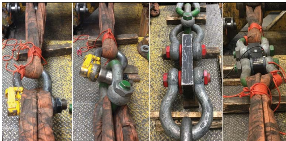
Figure 3: Systematic tests with load cells to evaluate the effect of misalignment
