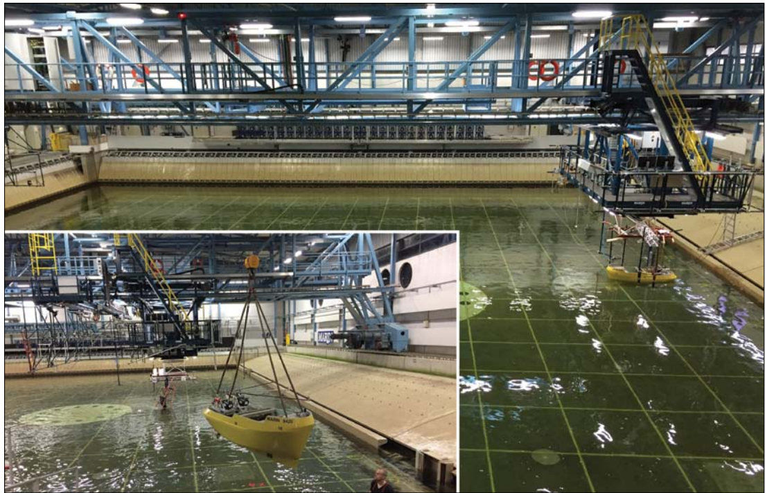
Figure 1: Model testing to investigate effect of water depth and line length in the MARIN offshore basin (lxb = 45x36m with movable floor 0-10m depth)
